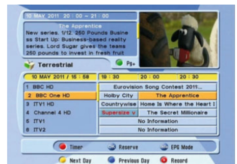
The EPG for DTT channels supports 7-day DVB data and can be used to schedule recordings. View what's on six channels or one at a time
