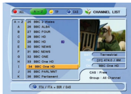
Channel lists can be sorted A-Z, by transponder or conditional access system and satellite and terrestrial lists viewed separately
